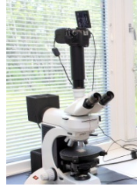
Polarization microscope with a digital camera connected to a PC work- station.
